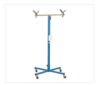
The SRDL Duct Lift is a great tool for safe and precise lifting of ducts. Now you don't have to be two persons when lifting a duct for installation. The duct lift can lift ducts of a maximum weight of 25 kilos to a maximum height of 3000 mm. The lean design of the duct lift allows you to easily move it around on and between building sites. You can even get it through doors as narrow as 700 mm. The duct lift is very easy to assemble and dismantle.
