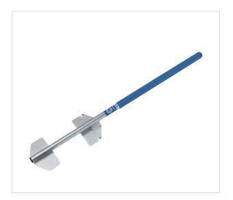
SRH is a carrying handle which makes it substantially easier to manually move circular ventilation ducts at the building site. The handle fit ducts Ø 315–1250, but it is adequate to limit its use to the sizes Ø 400–800. You ought not to exceed the recommended maximum carrying weight of 25 kg per person. One person at each duct end uses a handle each.
