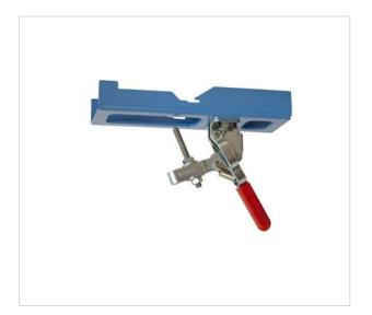
D3H is a helping tool to join rectangular ducts and fittings. The tool is clamped to the already mounted product. The tool carries the unmounted product's one end so you don't have to hold it yourself and also it guides the unmounted product in place so that the joining profiles are located at the right position. The tool only works at horizontal duct runnings. **NOTE!** The tool only works with products equipped with joining profiles type LS.
