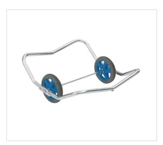
TRO is a trolley which makes it substantially easier and more ergonomic to manually move circular ventilation ducts and other heavy products at the building site. The trolley is suitable for ducts Ø 400–1250. Trolley with loaded duct is easily moved by one person. Maximum load: approx. 100 kg. Weight: 4,0 kg.
