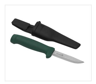
KNIFE is a sturdy and durably sharpened knife for tough tasks e.g. hole-making in ventilation ducts. The blade is manufactured of 3 mm Japanese carbon steel and sharpened with double edge angles. The handle and sheath are manufactured of extra impact resistant PP plastic.
