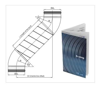
To make Offset calculations easier we have made a pocket guide. Instead of using your time to measure and test the duct length you can use your guide.
