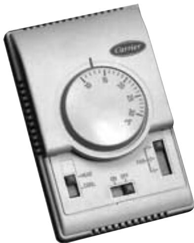
Elegant room thermostat, blending in with most room decors. Two models available: one with a manual heating (winter)/cooling (summer) selector, and the other with an automatic switch. Both are for 2-pipe, 2-pipe changeover, 4-pipe or 2-pipe plus electric heater systems.
