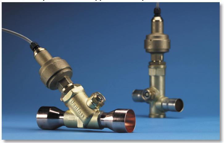
ETS is a series of electrically operated expansion valves for precise liquid injection in evaporators for air conditioning and refrigeration applications.
