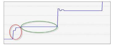
During the heating phase, the probe will not measure, it will keep the last measured value for the duration of the heating period. The steep rise (red circle) corresponds to the one-minute long measuring phase. The probe is then heated and cooled (green circle) over a period of five minutes. The probe must always be powered in order for the heating function to work correctly.
