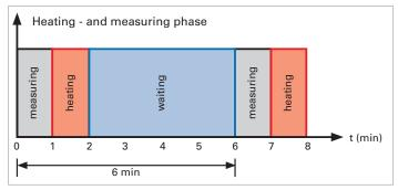
Current consumption rises up to 35 mA (at 3.3 VDC) during the heating phase. To ensure a correct heating function, 35 mA is required.
