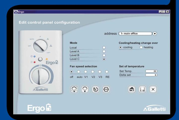
Via software it is possible to assign to the local user terminal, four different levels of function control. One of the must common possibilities is to fix via software the local room temperature set-point and the working mode, leaving to the user the choice of the fan speed and the variation (within a limited range) of the room air temperature around the set point.
