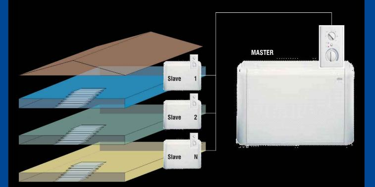
The installed microprocessor is the same as that used in the standard ERGO system. The "SMALL" solution is a master-slave system, in which up to 127 'MICRONET' control user terminals are connected together, one of which is assigned the role of 'MASTER'..
