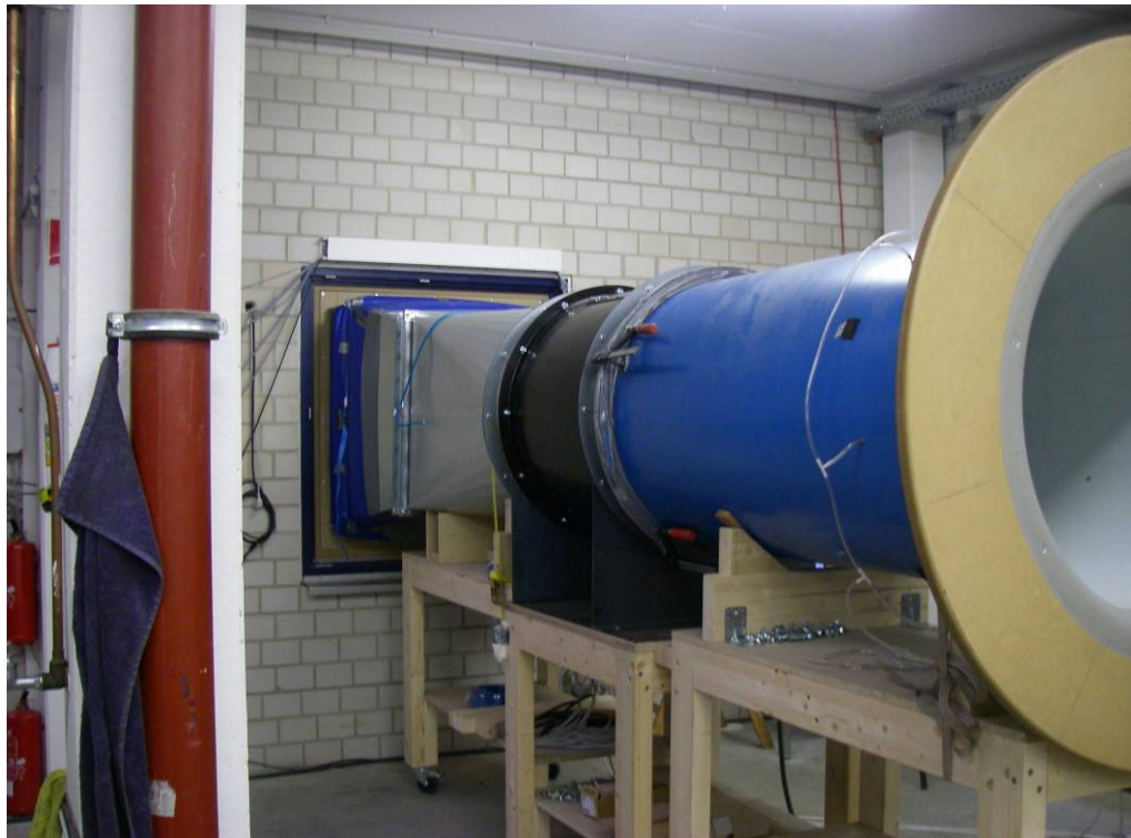
Fig. 2 Pressure differential system SAFETY WAY® supply air unit with volumetric flow measurement system in front of test room
