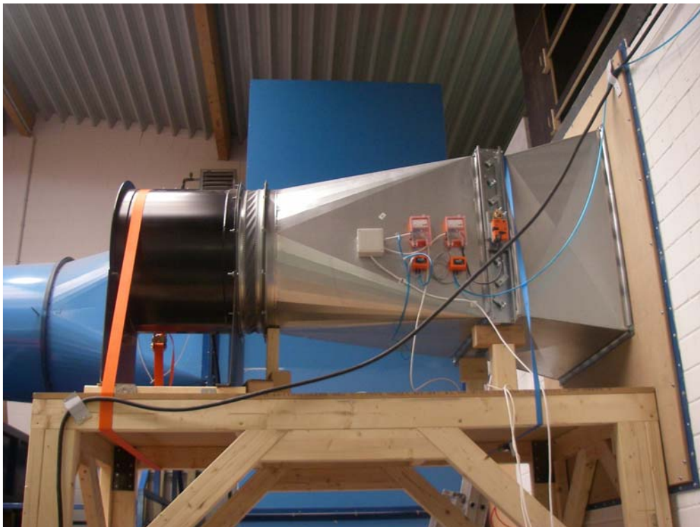
Fig. 9 SAFETY WAY® outlet air unit at test room
