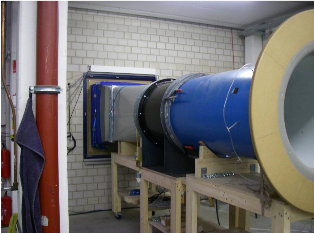
Fig. 1 Pressure differential system iSWAY-FC® with volumetric flow measurement system in front of test room
